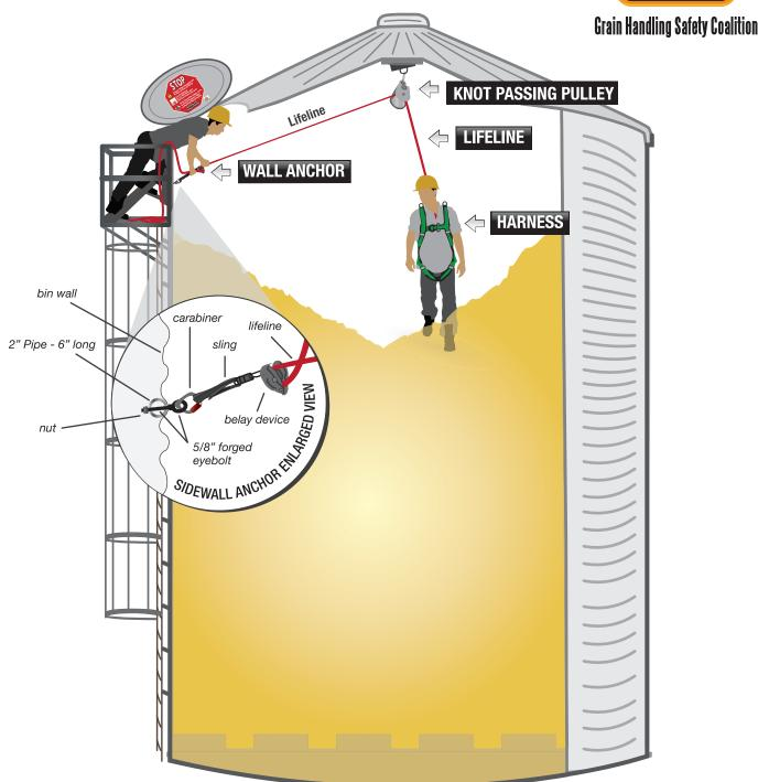
A sidewall anchor is NEVER attached to any part of the inside bin ladder. The inside bin ladder was omitted from this drawing for illustrative purposes. www.grainsafety.org
